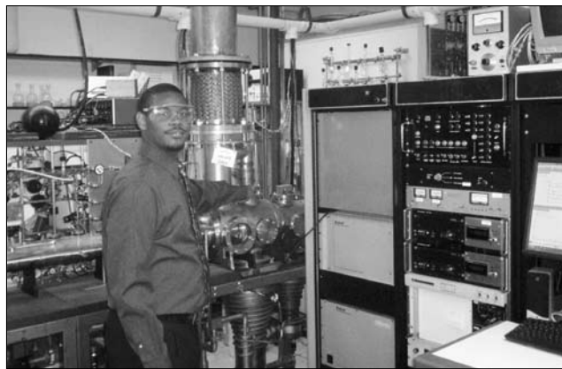
Mitchell Thompson, a FE-R student in Spring 2006, collecting data on the chemical reaction mass spectrometer in Professor J.J. Grabowski's lab.
