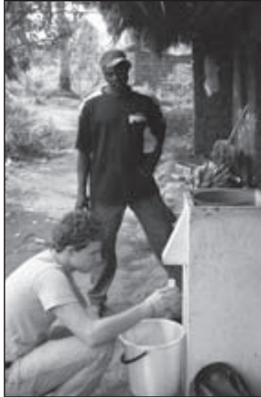
Hope College engineering student Mark Humberstone samples water from a Manz Biosand Filter in Nkuv, Cameroon, West Africa.
